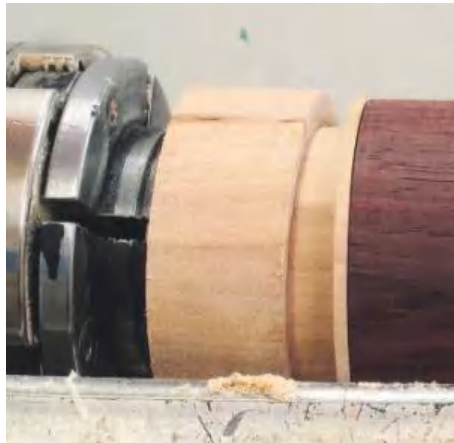
STEP 23. Mount the other piece of apple in the chuck and then cut a spigot that will fit snugly into the base. I like to make the fit so it goes on easily but with no sideways movement
